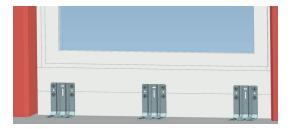
**Note:** The number of MUNTADO depends on the size of the floor deep window- or door element. The weight of the window- or door element must be absorbed by supporting and spacer blocks (not included in scope of delivery) on the underside of the window/door
