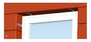
**Note:** The weight of the window must be absorbed by supporting and spacer blocks (not included in scope of delivery) on the underside of the window
