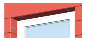
**Note:** The number of THERMINATOR depends on the size of window - the distance between the THERMINATOR may be a maximum of 700 mm for PVC windows. The weight of the window must be absorbed by supporting and spacer blocks (not included in scope of delivery) on the underside of the window.
