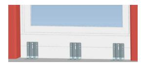
Note: The number of MUNTADO depends on the size of the floor deep window- or door element. The weight of the window- or door element must be absorbed by supporting and spacer blocks (not included in scope of delivery) on the underside of the window/door
