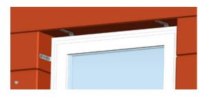
**Note:** The number of INVADI depends on the size of window - the distance between the INVADI may be a maximum of 700 mm for PVC windows. The weight of the window must be absorbed by supporting and spacer blocks (not included in scope of delivery) at the underside of the window.
