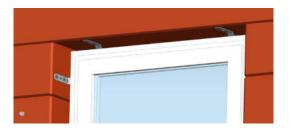
**Note:** The number of ENBATI depends on the size of window - the distance between the ENBATI may be a maximum of 700 mm for PVC windows. The weight of the window must be absorbed by supporting and spacer blocks (not included in scope of delivery) on the underside of the window.
