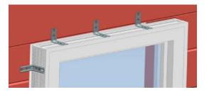
**Note:** The weight of the window must be absorbed by appropriate structural measures / suitable brackets or similar (not included in the scope of delivery) on the underside of the window
