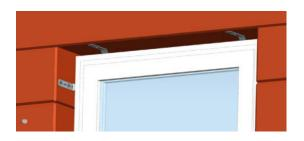
**Note:** The number of ALUMINIO depends on the size of window - the distance between the ALUMINIO may be a maximum of 600 mm for PVC windows. The weight of the window must be absorbed by supporting and spacer blocks (not included in scope of delivery) at the underside of the window.
